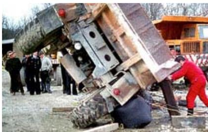
Thereby the tactic used is a relatively simple one: Stepwise lifting - first creating the necessary space with a small LAMPE-LIFTER and then pushing the load with a larger device over the centre of gravity.
