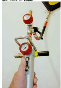
• The new inexpensive pressure control fitting can be used for filling by means of the control fitting, and it can then be removed. This means that an optional number of LAMPE-LIFTERS can be employed with minimal technical effort.
